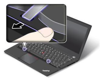
6. Adjust the keyboard frame in place with the keyboard multi-tool and ensure that all the latches are secured under the keyboard bezel.
